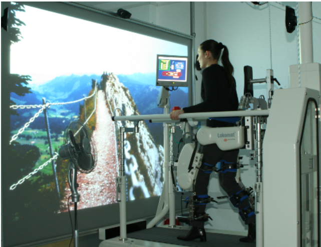
Fig. 2 Lokomat equipped with a multimodal display comprised by a stereo projection system, a doubly surround sound system, a wind-generating fan, and the Lokomat providing haptic feedback. Virtual objects can be projected motivating the patient to lift the leg.
